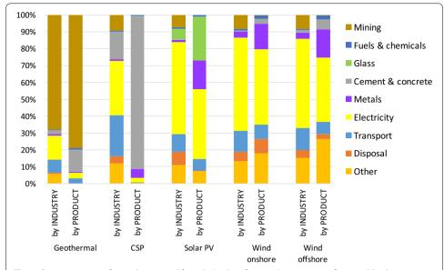
**Fig. 5** Decomposition of greenhouse gas life cycle (carbon footprint) inventories of renewable electricity generation technologies by industry (*left column*, cf. Wolfram et al. 2016) and by product (*right column*, this work). *CSP* concentrated solar power, *PV* photovoltaic
