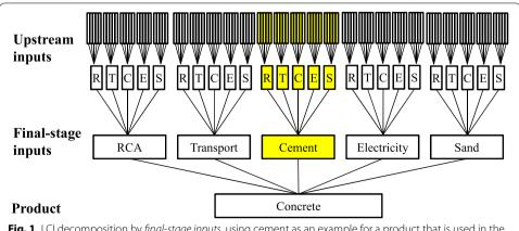
**Fig. 1** LCI decomposition by *final-stage inputs*, using cement as an example for a product that is used in the final stage of producing the product for which an LCI is undertaken
