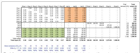
**Fig. 4** Example transaction matrix with eight processes, three industries and five product sectors with extensions for greenhouse gas emissions (upstream and downstream cut-off matrices are shaded in green and orange, respectively)
