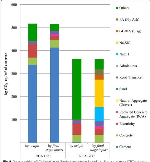
**Fig. 8** Decomposition of LCIs by *origin* and by *final-stage inputs* for ordinary Portland cement (OPC) concrete and geopolymer concrete (GPC)
