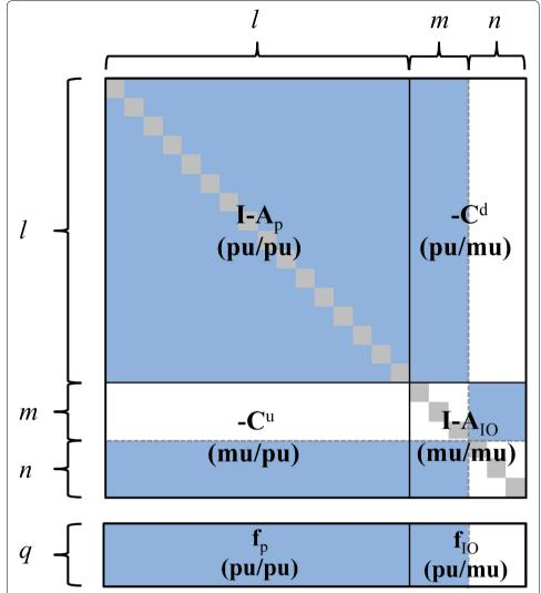
**Fig. 3** Integrated coefficient matrix ( $\mathbf{I} - \mathbf{A}_{|H}$ ) of integrated hybrid LCA (blue-shaded areas include nonzero values, but may be sparsely populated; non-shaded areas contain zeroes; gray-shaded areas represent 1s on the diagonal; pu physical units; mu monetary units)
