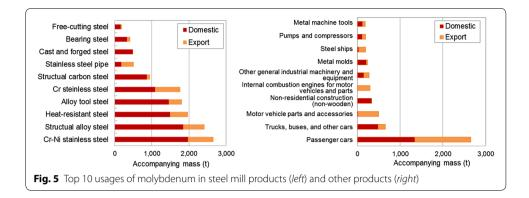
was highly concentrated into automobile-related products (Fig. 5, right-hand side). As a consequence, 7.7 kt (27% Mo derived from imported virgin sources) of molybdenum was exported with products. Exported molybdenum in raw materials was 0.8 kt.
