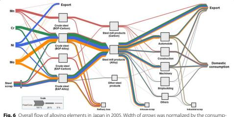
**Fig. 6** Overall flow of alloying elements in Japan in 2005. Width of *arrows* was normalized by the consumption of each alloying element in steelmaking
